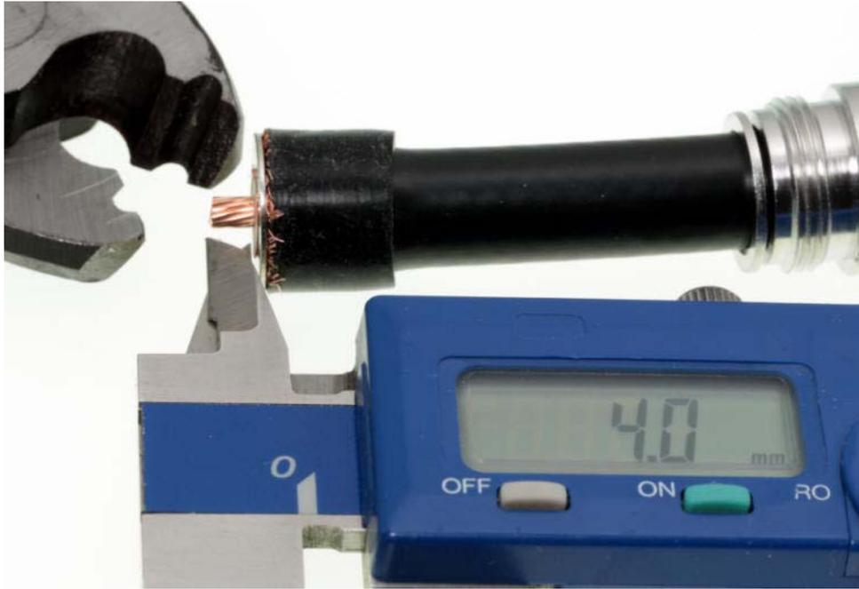
Our coax cable scissors cut the center conductor in a way that its structure does not change. You can easily put the center pin onto the cable.
